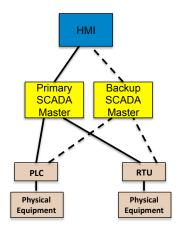
Fig. 1. Conventional SCADA system architecture.
